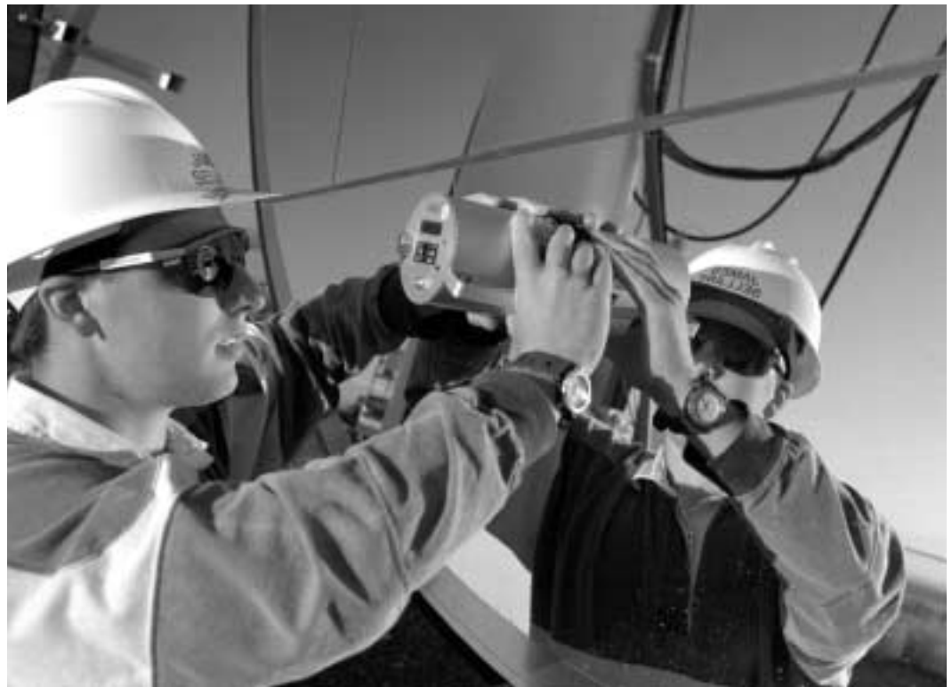
A technician measures mirror surface quality on a dish concentrator.
