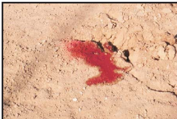
Figure 4-3. Husky ink-mark indicating metal below the surface
